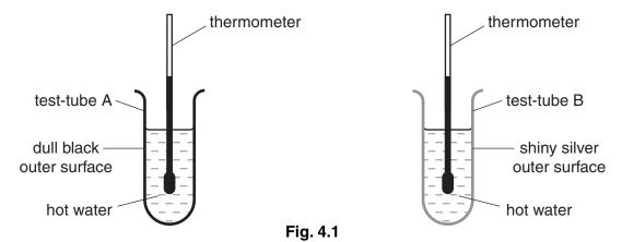
Test-tube A has a dull black outer surface and test-tube B has a shiny silver outer surface.
